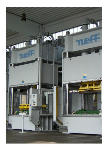
4SP 160: 4-Column press 160 t and 400 to pressure performance for production of automotive parts
