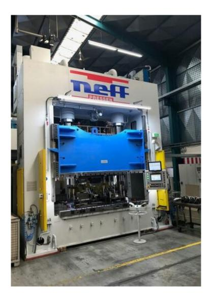
DZP 800 to with 4-point cutting impact dampening and ram –skewing monitoring for production of automotive parts
