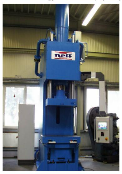
EZP 160: Single column deep-drawing press 160 to. with 4-fold guided ram plate and tool clamping system
